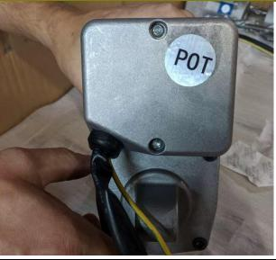
For new Landice units, the elevation pot key will be located in the motor pan, as shown above. If replacing an elevation motor on an older unit, the key will be bound along the grounding wire. **NOTE:**Needle nose pliers can be used in the event the pot key is lost. Remove the POT sticker to expose the elevation pot and proceed to the next step.
