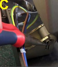
Using your screwdriver, remove both screws as shown in Figure A. Next, use your needle nose pliers to remove the two elevation pins connecting the nut to the elevation legs. Now use the pliers to remove the clevis pin, as well as the clevis bolt. A rubber mallet will help you replace the clevis bolt. You should now be able to completely remove the elevation motor from the unit. To re-install, follow the directions in reverse. Proceed to the next page for Calibration Instructions.
