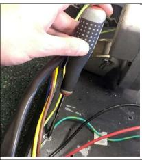
Begin by using a block of wood or something sturdy that can be propped underneath the motor pan. You will then power down the unit, and unplug from the power source. Next, locate the elevation harness and unplug from the lower board. Finally, use your screwdriver to remove the grounding wire.
