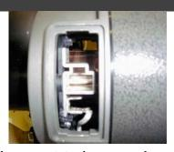
The commutator is copper color and shiny. Cleaning the commutator with a cleaning stone or piece of emery cloth may remove the dull appearance & black scorch marks.
