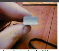
A good motor brush will be shiny. Free from scorch marks, chips, and not dull where the commutator would make contact.
