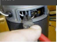
Take a needle nose pliers and use them to remove the motor brush wires from the connector
