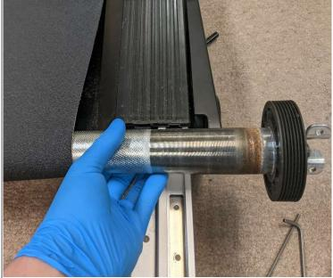
Once the bolts are removed, you are now able to remove the entire motor pan from the machine. From here, you can simply remove the **drive belt** and/or **front roller** and replace if necessary.
