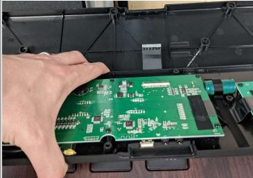
Begin by using your Phillips head screwdriver to remove 12 screws from the back of the display. Remove the back panel to reveal upper circuit board.
