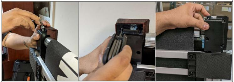
It is helpful to lean the unit up against the wall for this installation. Begin by using your **6 mm** Allen wrench to remove the tensioning bolt on either side. Next, use your **4mm** Allen wrench to remove 4 bolts keeping the rear bottom end cap in place. Next, remove both the front and bottom end cap components.
