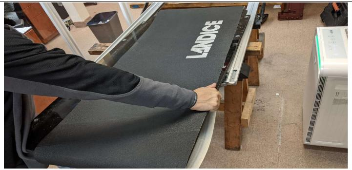
Next, flip the treadmill back over to its normal position, face up. You can now remove the deck and treadbelt from the frame of the unit, and slide the treadbelt off the deck.
