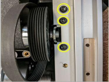
Using a 4mm Allen Wrench, continue removing all the bolts circled above.
