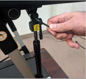
Using your Allen head wrench, remove the M5x10 Allen head shoulder screws as shown above.
