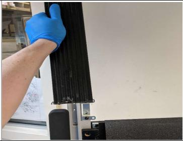
Begin by folding the arms down on the machine flat, and then propping the treadmill up against a wall, rear roller side up. Slide the side frame covers up and off the unit.
