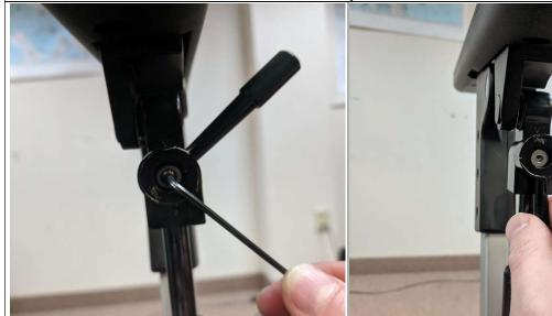
Using a 1/8" Allen wrench, remove the bolt and bolt washer, that was previously hidden by the sticker. Then remove the lever. PLEASE NOTE: You will need to use the same Silver washer and Bolt Washer, so make sure you put them in a safe place.
