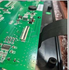
Locate the ribbon connection that leads to the button panel. Using your finger, nudge the black tab into the upward position, as shown above. You will then be able to remove the ribbon from the membrane. Next, remove the entire upper display assembly from the treadmill. To replace, follow the instructions in reverse.
