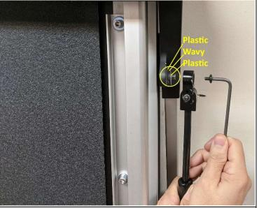
You can now remove the strut from the machine. It may be helpful to unlock opposite strut and rotate upright assembly up and down to aid with strut replacement. The new strut is shipped slightly compressed to aid with installation. Be careful to keep the washers in place as you replace the strut.
