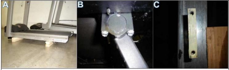
Begin by unplugging the treadmill from the wall outlet. Place the treadmill on wooden blocks to relieve pressure on the elevation leg assembly (**Fig. A**) Next, using your cordless drill and Phillips bit, remove the screws from the bearing block (**Fig. B**) Apply a thin coat of Lubriplate grease on the inside and top surface of the bearing block.(**Fig. C**)
