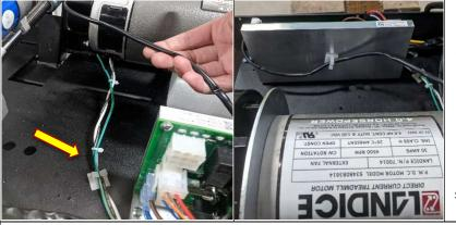
Braid the White/Black motor wires and secure it to the motor pan. Then route the drive motor wires to the lower board, ground the green wire to the motor pan. Route the Speed Sensor wire along the back of the lower board, securing it in the clip, or with electric tape to the back of the lower board.
