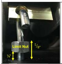
The drive belt tensioning nut is located underneath the motor pan, connecting the J-hook to the motor bracket. Make sure the plastic washer is in place, prior to tightening. When tightening the tension of the nut, it will pull down on the motor bracket while tensioning the drive belt.
