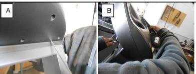
**STEP#1:** Insert a long push rod or Phillips head screw driver (approximately 16" long) thru the access hole on bottom back of HTEC assembly. (FIGURE A). Grab the panel and pull it away from the HTEC assembly once the push rod pops the panel off the Velcro seal from the top (FIGURE B).
