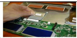
**6:** Take the membrane ribbon cable and connect it to the pins on the upper board.
