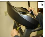
**#1:** Insert a long push rod or Phillips head screw driver (approximately 16" long) thru the access hole on bottom back of HTEC assembly (FIGURE A). Grab the panel and pull it away from the HTEC assembly once the push rod pops the panel off the Velcro seal from the top (FIGURE B). Disconnect console from Wire harness and follow instructions to replace parts as necessary.
