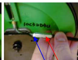
Figure D Loosen the locking nut for the turnbuckle. To remove slack, turn the buckle clockwise. To obtain slack turn it counterclockwise.
