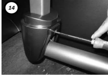
14 Install the Knuckle Covers. Use 2 phillips screws (K) to secure both sets of covers.
