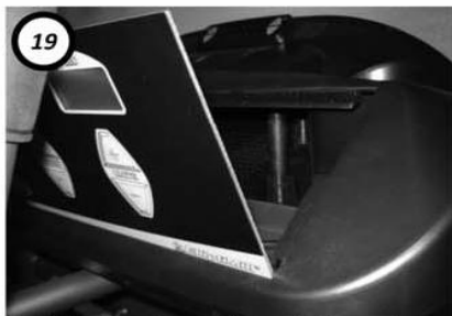
19 Carefully place the membrane in the control panel Pod (don't scratch plastic edges) tilting it towards you so you can make all connections.
