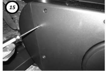
15 Install the Base Endcaps using 4 phillips screws (I) for each.
