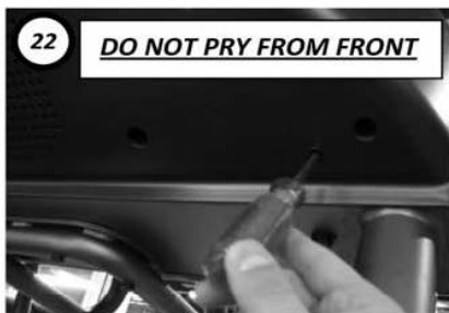
22 DO NOT PRY FROM FRONT Press membrane into set position. If you need to free the membrane, use a long screw driver to pop it out from back using the access hole.
