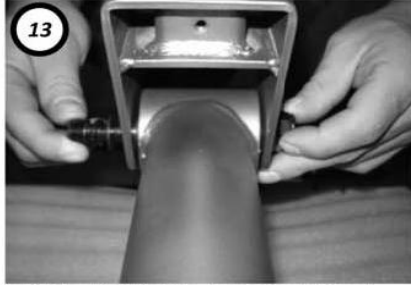
13 Install the Foot Pedals. Use a socket head cap screw (F), spring washer (Q), flat washer (N) and nylon lock nut (M) for each pedal.
