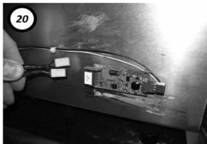
20 Connect the 2 heart rate cables to the 2 side by side 3-pin connectors on the small PC board on the far side of the membrane.
