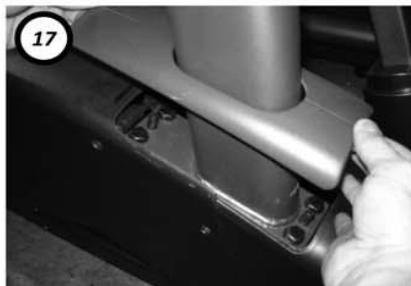
17 Install the Upright Mount Covers. Screw the outer and inner pieces together trapping the upright and slide them down until they click.
