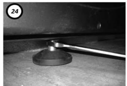
24 Check stability of unit by verifying that all leveling feet are pressing against the floor.
