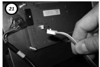
21 Connect the upper harness from the upright to the edge connector and the accessory harness coming from the POD to the 3-pin connector.
