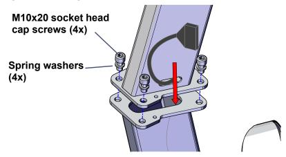
3. Connect main power harness from upright bike base to intermediate harness located inside the upright tube (Figure 3-2).
