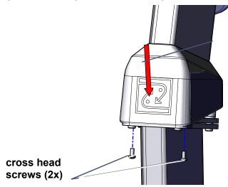
6. Install Bottle Holder onto upright tube. Secure with (4) #21 M5x15 cross head screws (Figure 3-4).
