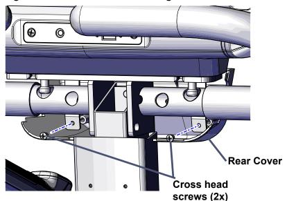
10. With rear cover in place, position front cover so both plastic mounting inserts go through the cross bar access holes. Secure with (2) #25 cross head screws. Do not over tighten or plastic components may be damaged (Figure 2-6).
