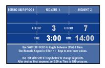
Note: Press SWITCH FOCUS to toggle between effort and time values for the current segment. To change segments, press NEXT SEGMENT or PREVIOUS SEGMENT. You can change segments in either the forward or reverse direction.
