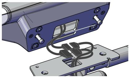
Rotate console upward, while carefully routing wire connections into base tube and/or console (Figure 2-4).
