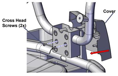
Figure 2-9. Rear Seat Back Cover Installation
