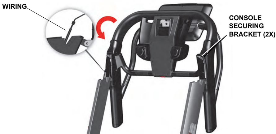
Figure 2-18. Lower Handrail/Console Assembly into Place
