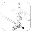
2. Attach the pannier rack to each of your rear drop outs using two of the M5 screws, washers and nuts provided.
