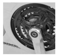
Your left hand shifter (L) has numbers 1-3. This moves the chain up and down the three chainrings. There are two "triggers" on the shifter. Your thumb moves up from L1-L3. Your index finger moves down from L3-L1.
