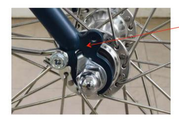
Important! If you have tabbed washers put the tab into the hole in the fork. Check the wheel is sitting centrally in the fork before securely fastening the wheel nuts with the 15mm spanner.
