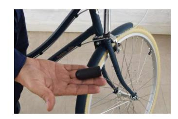
Remove and keep the little plastic plug (if there is one) from the head of the stem top bolt
