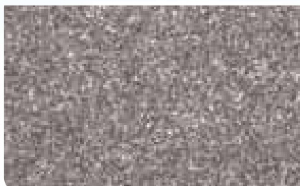
ultrafine grain size carbide material used to reach both hardness and toughness
