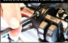
Remove OEM Throttle Grip -Throttle Tube from handlebar
