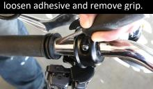
Clean residue from handlebar and slide Lock-On Clutch grip onto bar.
