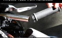
Loosen throttle cables to alleviate cable tension.
