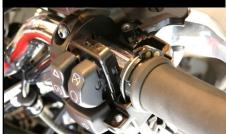
Loosen front brake perch TORX bolts and slide away from housing.
