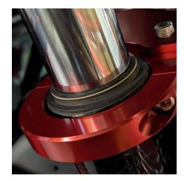
Install you're your fork tubes back onto the bike. Make sure to have the tubes push down fully to get maximum travel. This will give enough travel for the brace to not hit the lower tree trim cover. <u>This kit will NOT fit lowered forks.</u> Re install your front wheel & fender.
