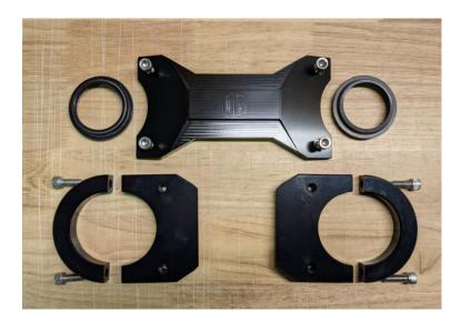
2. Once you have your fork tubes in hand. Slide in the supplied 49mm Dust Seal Covers. Tap these in so they sit flush using a seal driver. These refer to picture below.
