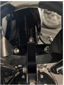
6. Install your fairing shell onto lower and upper fairing mounts using supplied ¼-20 hex bolt (4x), locknut (4x) & washers (8x – one on each side). The fairing shell brackets (Left & right) go on the inside of the upper & lower fairing mounts. Put the nut on, facing the rear of the bike. Also be carefull not hitting your tank with your key/ratchet while you thigh it down. Recommended Torque 15 ft-lbs.
