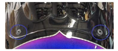
12. Using some blue threadlocker, pre install through your windshield the upper windshield hardware so it hold onto the screen with the supplied rubber washers in the back of the shield. Refer to pictures below.
