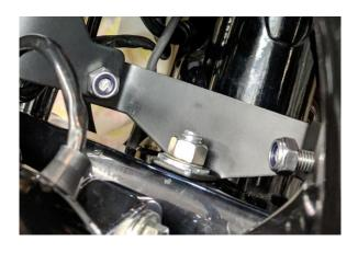
7. Install your fairing shell onto lower and upper fairing mounts using supplied ¼-20 hex bolt (4x), locknut (4x) & washers (8x – one on each side). The fairing shell brackets (Left & right) go on the inside of the upper & lower fairing mounts. Put the nut on, facing the rear of the bike. Also be carefull not hitting your tank with your key/ratchet while you thigh it down. Recommended Torque 15 ft-lbs.
