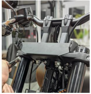
Install the supplied headlight bracket kit under your lower triple tree & your lower fairing bracket on top of it according to pictures below using supplied hardware. Lock it down tight by hand. Refer to picture below.
