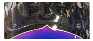
13. Using some blue threadlocker, pre install through your windshield the upper windshield hardware so it hold onto the screen with the supplied rubber washers in the back of the shield. Refer to pictures below.
