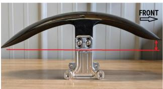
3. Install your fender kit onto the forks lowers using OEM hardware (4x screws). Just thread the bolts in so the fender hold onto the bike. At this point you want to adjust the fender clearance & angle by pulling onto the fender so it move within the adjustment. Once you are happy with the fitment/adjustment, remove the fender gently from the bike by removing the OEM hardware (4x screws).
