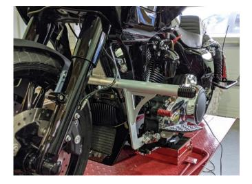
6. **IMPORTANT STEP:** Before going out for a ride with your new crash bar, you must tie down your bike and compressing the front end to ensure there is no contact between your front fender and the crash bar. If there is contact between fender and crash bar please contact us
