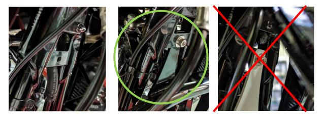
3. Assemble the Clutch side / Left side first. Placing the supplied billet washer/spacer between the frame & the crash bar (refer to picture below) use the supplied 3/8-16 x 1 1/2" screw, washer & lock washer to bolt the bar onto the lower frame support. DO NOT TORQUE IT YET. Repeat on the Throttle side / Right side of the bike.
