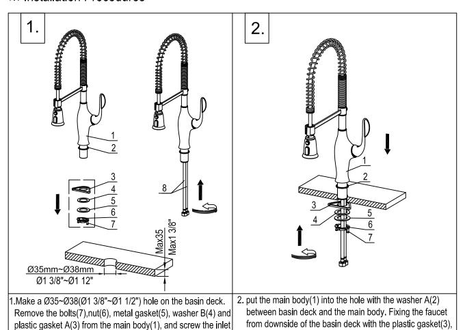
washer B(4), metal gasket(5), nut(6) and bolts(7).
