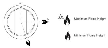
Maximum temperature setting/recommended control knob position for burner ignition.
