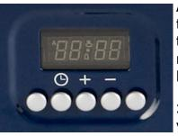
After you have pressed the clock button once, you can then immediately set the minutes by using the plus button +. If you enter an incorrect time you can use the minus button - to correct the time. Press and hold the clock button  $(\Box)$  until the LED display flashes to set the hours.
