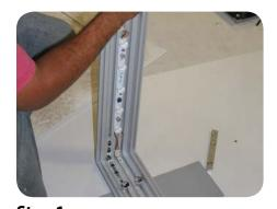
**Step 1:** Start by placing the light strips on the inside groves of both sides of the Mammoth Frame. Place the strips so that the "male" connections are on the bottom of the light strip with the "female" connections at the top of the light strip.
