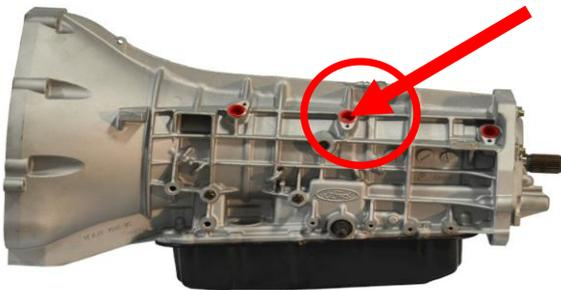
After installation, remove the 5/16" hex plug (this is the fill plug).
