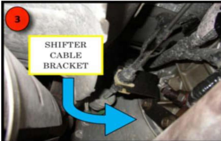
If alignment cannot be achieved, verify that the shifter cable bracket is not bent or out of position. Check the witness marks where the bolts go through the bracket and line the bracket up to that.
