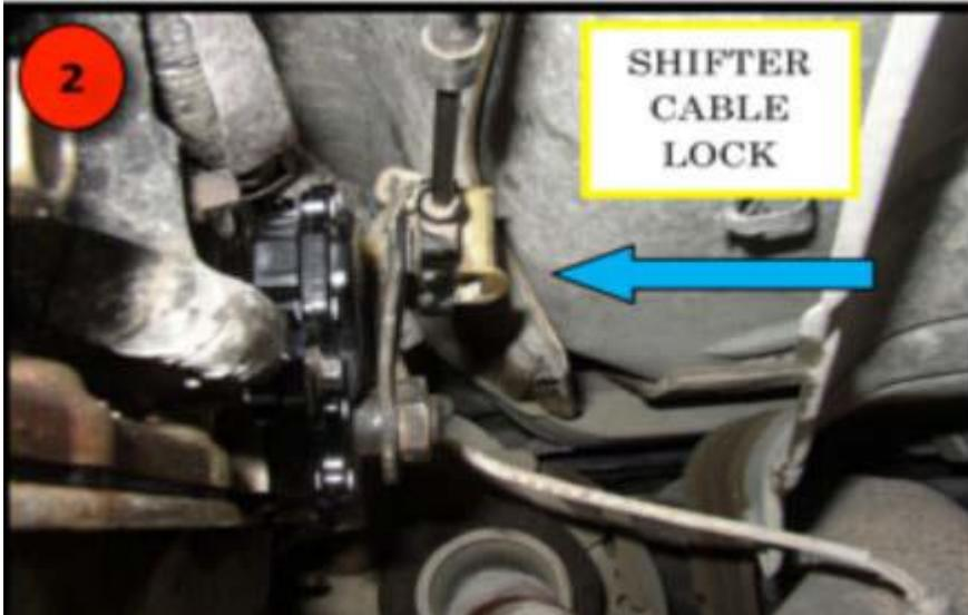
Verify the shifter linkage is lined up properly through each range. If not, place the shifter in the manual low position on the column. Pop the shifter cable off the manual arm on the transmission. With a pick, pull the lock tab toward the outside to release the lock and slide the tab up. Move the lock and center it onto the manual arm ball. Snap the lock onto the ball and slide the lock tab down. Move the shifter handle into the neutral position and verify alignment.
