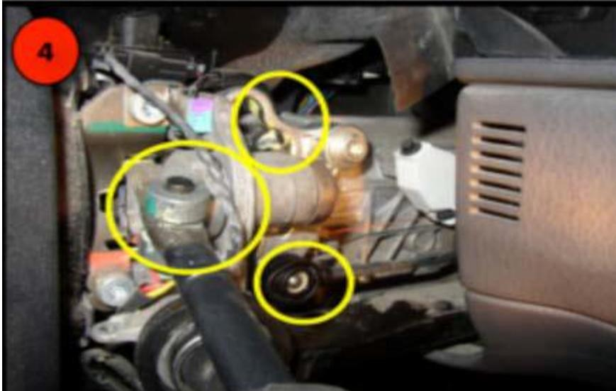
Make sure the alignment marks are aligned. If the adjustment is even slightly off, the computer will read a reverse signal and boost line pressure before the manual valve is moved into the reverse position.
