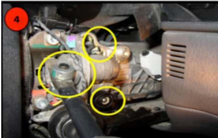
If the alignment still cannot be achieved, inspection of the column itself may be needed. There should be no slop felt while moving the shifter handle. If there is, either the shifter cable is stretched or the shifter mechanism is worn out. At this time, you cannot purchase any of the shifter mechanism parts separately; you have to buy a column kit.
