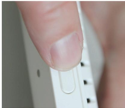
**2** Push and hold the standby button located on the right side of the panel for 3 seconds.
