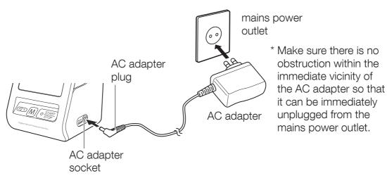
**2** Plug the AC adapter into a mains power outlet.
