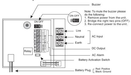
\*Battery activation switch is just for no AC input. If with AC input, when AC off, the unit can switch to with battery powered automatically, no need to press this button.
