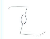
In line loops are used to enhance the level of security offered by an electric fence by detecting attempted separation of fence wires. By creating a connection between 2 earth wires and leaving just enough room for natural movement of the live wire, the alarm will sound as the live wire touches the in line loop.
