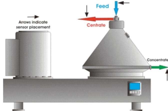
A common position of a Solids Sensor is on the **Centrate line**, helping with separator control ensuring performance optimisation and identifying any higher than desired solids concentration.
