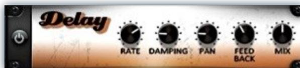
**Feedback** - This knob controls the feedback of the delay effect. High values can cause an endless loop.
