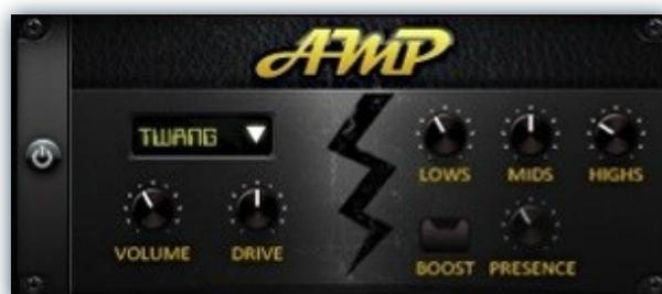
**Highs** - This knob controls the gain of high (treble) frequencies.
