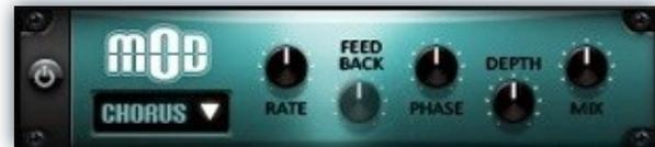
**Depth** - This knob controls the depth (intensity) of the selected effect.
