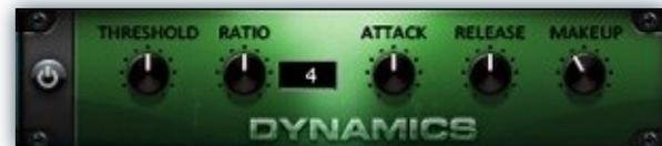
**Release** - This knob controls the release time of the compressor.
