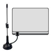
The iFUEL® TANK comes with a passive internal GSM antenna (SMA connector) on CON6. However, if the device is mounted inside a metal enclosure, it might be hard to obtain good reception. In such cases, connect an external GSM antenna, run the cable through one of the glands at the bottom of the casing, and make sure the antenna itself is located as high as possible to ensure good mobile reception.
