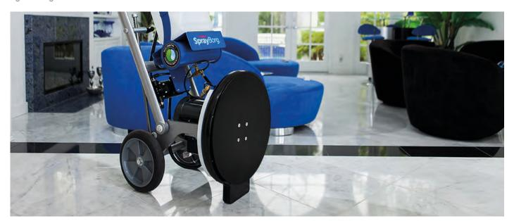
**STEP 1 Pad** - Removal of deep scratches and to resurface the stone flooring. Step 1 is the most important step to achieve the best results. Step 1 will grind the floor down and allow for steps 2-5 to achieve a high gloss result.
