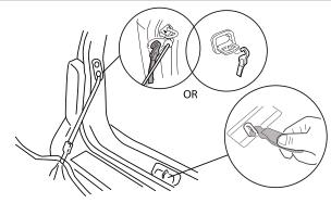
From inside the tent, find the center strap and attach the hook to the middle tailgate latch. Secure the two side straps to either the the cargo bay area hooks or the tailgate latch
