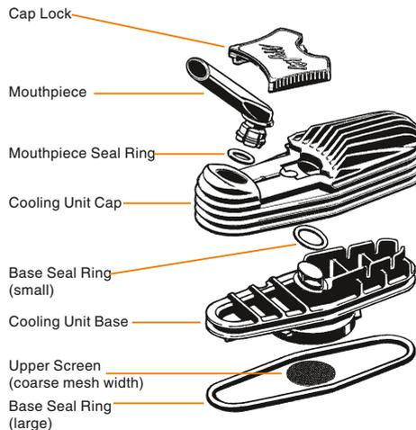
**10.1. Disassembling and Reassembling the MIGHTY Cooling Unit**
