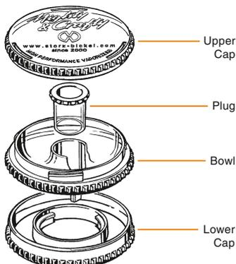
To fill the Filling Aid, remove the upper cap and fill the bowl incl. plug with ground plant material. Replace the upper cap and close it.
