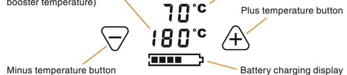
The temperature can be set between 40°C and 210°C (104°F and 410°F) (see Section 4. "Overview of Plants").
