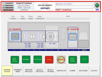
**System ID** – Displays the serial number of the OnTrak, or can be configured with a user system ID.
