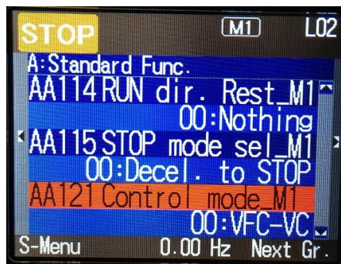
Figure 31: Motor Control Mode
