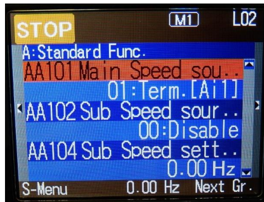
Figure 28: Main Speed Source
