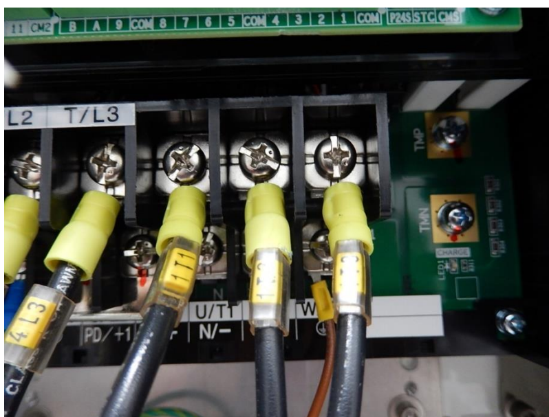
Figure 12: 3-Phase Motor Output Connection
