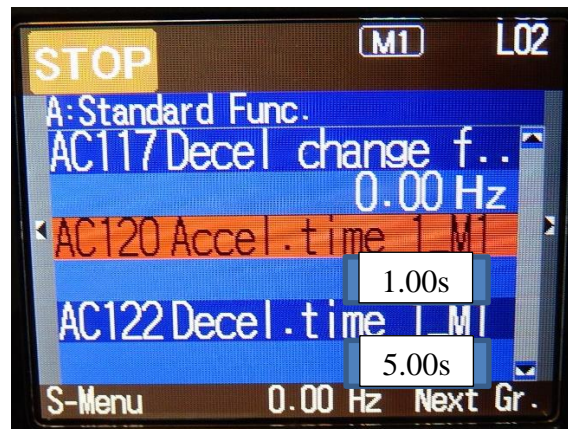
Figure 39: Motor Acceleration & Deceleration Time
