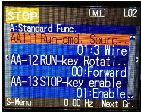
Figure 30: Run Command Source
