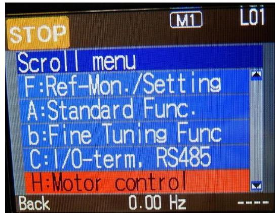
Figure 37: Motor Parameters Selection
