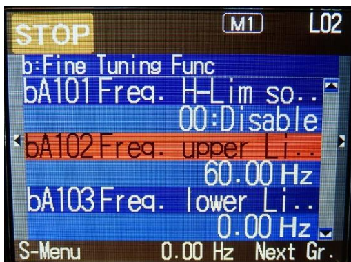
Figure 34: Upper & Lower Frequency Limits
