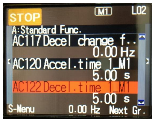
Figure 32: Motor Acceleration & Deceleration Time
