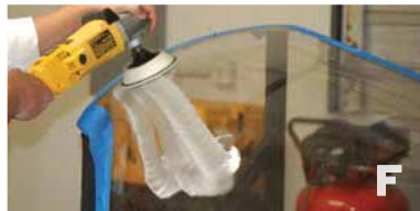
Slowly activate tool and maintain medium contact pressure between disc/pad and contour of surface.
