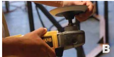
Attach backing plate to tool. MAJOR: Either curved or flat surface backing plate from Major Restoration Starter Kit. MINOR & FINISHING: Select either 3" or 6" size backing plate.
