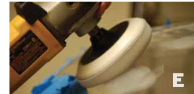
Compress disc/pad against surface and work polish into disc/pad to minimize overspray.
