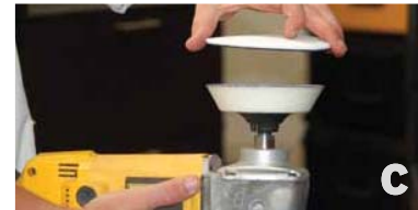
Center and velcro restoration disc or pad to back plate. Re-center if disc/pad spins unevenly.
