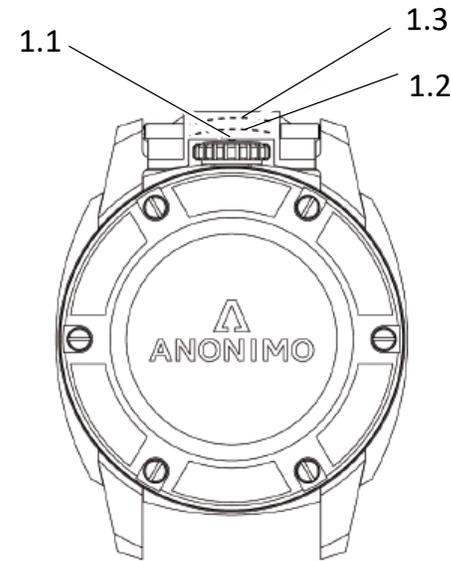
**Position 1.1:** The watch water resistance is guaranteed. The crown is locked by the patented protective lever integrated into the watchstrap. In this position, the watch can be wound manually after unlocking the crown. (See “Getting started”).
