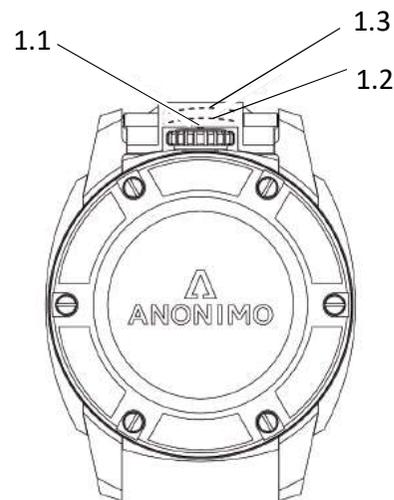
**Position 1.1:** The watch water resistance is guaranteed. The crown is locked by the patented protective lever integrated into the watchstrap. In this position, the watch can be wound manually after unlocking the crown (see "Getting started").
