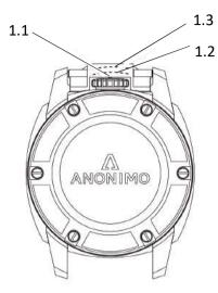
**Position 1.1:** The watch water resistance is guaranteed. The crown is locked by the patented protective lever integrated into the watchstrap. In this position, the watch can be wound manually after unlocking the crown (see "Getting started").
