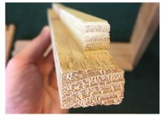
The shallower L bar makes a handle and structure support.
