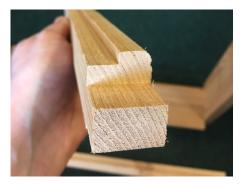
The flat side panel fits into the grooved side panel. The top aligns with the shallow L bar, at the top, and pokes out at the bottom.
