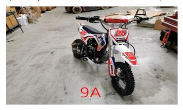
10. Fill petrol into the tank (Unlead 91, no Octane or E10), check the engine oil level, , key is on, kill switch is on, then kick it to start/press start button.(please let choke on for cold day). Helmet/long sleeves/long pants/enclose shoes are required.
