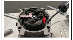
1. Use a screw driver try to take the clutch !!! Please Make Sure the Washer has been put aside!!!
