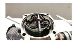
After you successfully complete up steps. You shall have a long shaft bolt and center washer out.
