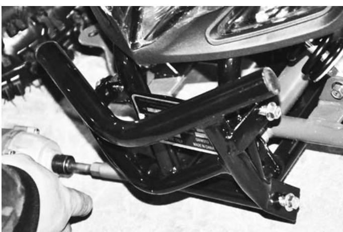
Step 3: Install front bull bar
