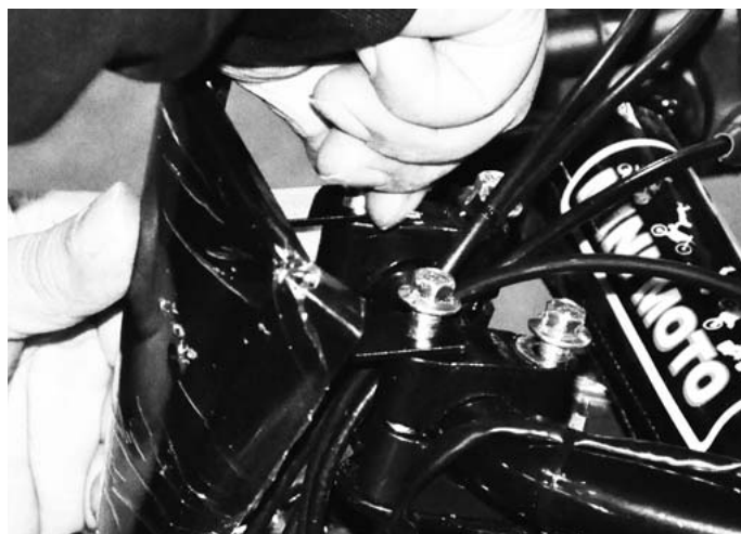
Step 2: Mount the handle bar to the ATV (Some of Model will have number plate)
