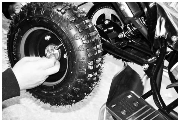
Step 6 : Mount the rear wheels and Rubber Dust Proof Covers
