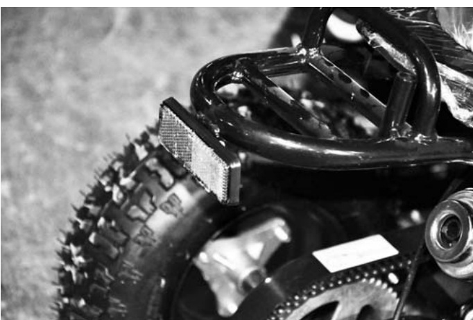
Step 5: Mount the Rear Reflection Plate on Rear Rack. For some of the model the reflection plate installed on side of the rear rack
