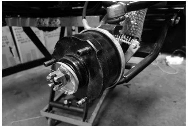
Step 7 : Undo the axle nut and remove the front wheel hub. insert the drum brake assembling to the stub axle and retighten the axle nut.
