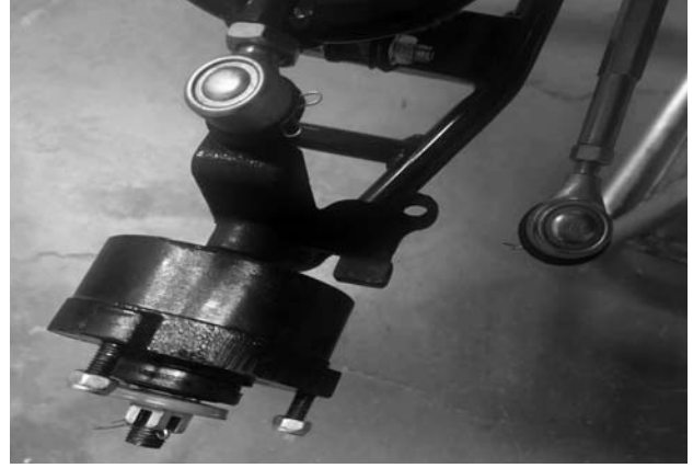
Step 6: Mount the front ball joint arm to the front stub axle for both side
