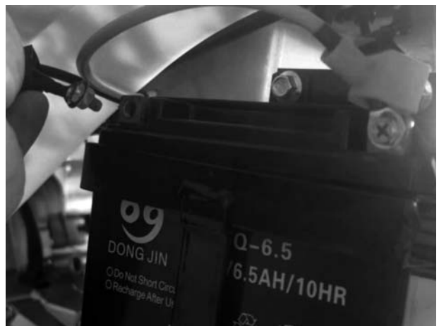
Step 8 : Access the battery from side of rear wheel. Connect the negative lead to the battery
