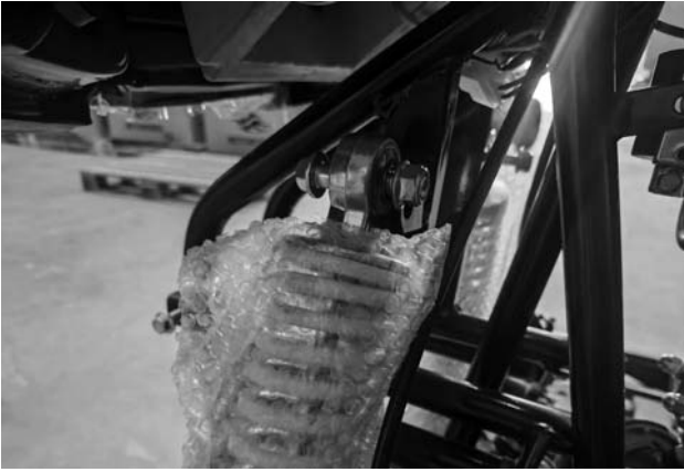
Step 5: Mount the top end of front shocker to the frame for both side
