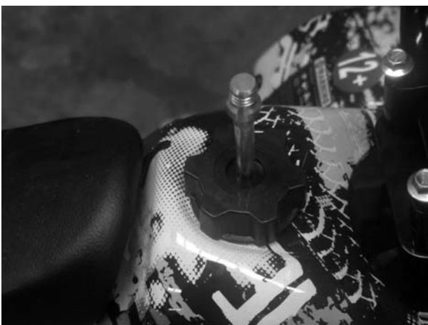
Step 9: Install the breath hose on the fuel cap
