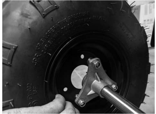
Step 6: Use provided bolts and nuts complete rear wheel installation
