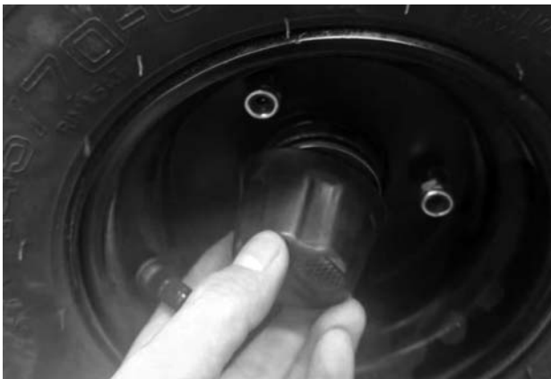
Step 8 : Mount the wheel to the hub with provided nuts for both side
