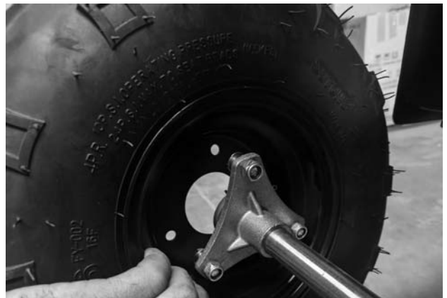
Step 9 : Mount the rear wheel to the rear axle with provided bolts and nuts
