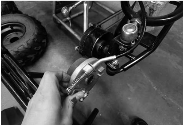
Step 7 : Undo the axle nut and remove the front wheel hub. insert the drum brake assembling to the stub axle and retighten the axle nut.
