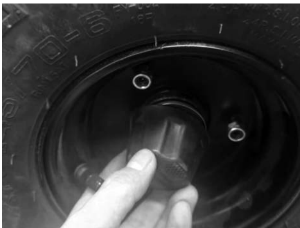
Step 7: Put on provided wheel cap to cover 4 wheels axle nuts
