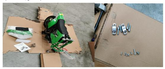
1, Install handlebar (4 bolts with brackets). See pic 1.
