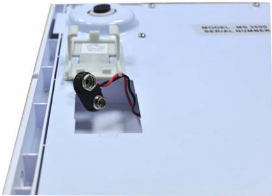
The scale uses 9V battery.
