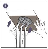
Press on the lower part of the sleeve firmly.
