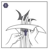
Cut the cable at an angle and pierce through the membranes of the sleeve.
